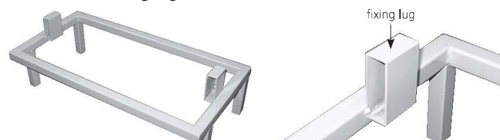
Stand to Locker Fixing Lugs (detail inset)
